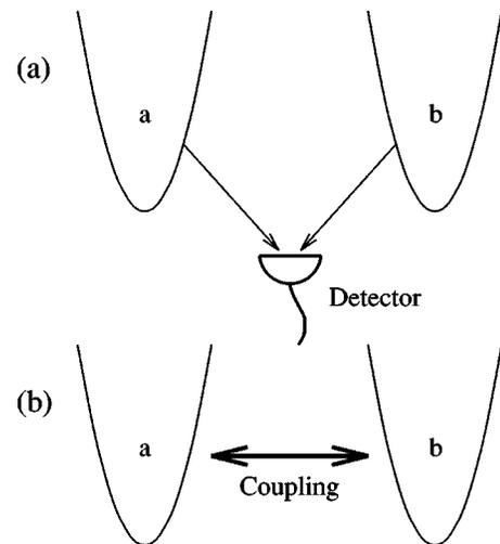
FIG. 1. Two methods of establishing a phase between the condensates. In (a), atoms from both condensates are allowed to fall onto a detector. An entanglement and relative phase arises since we cannot know from which condensate a detected atom has come. In (b), the two condensates are entangled by coupling them with Raman pulses for a time  $t = \pi/4\Gamma$ .
