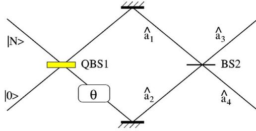
FIG. 1. (Color online) A schematic of a Mach-Zehnder interferometer with one quantum beam splitter (QBS1) and an ordinary 50:50 beam splitter (BS2). The quantum beam splitter has the property of creating a superposition of the form of (1) with all the particles in one output port and all in the other. There is a phase shift,  $\theta$ , on one arm that we wish to measure.
