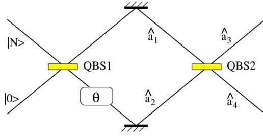
FIG. 2. (Color online) A schematic of a Mach-Zehnder quantum interferometer composed of two quantum beam splitters (QBS1 and QBS2). By feeding  $N$  particles into one input and 0 into the other and then detecting the particles at the two outputs (corresponding to the annihilation operators  $\hat{a}_3$  and  $\hat{a}_4$ ), Heisenberg limited measurements can be made of the phase shift,  $\theta$ .
